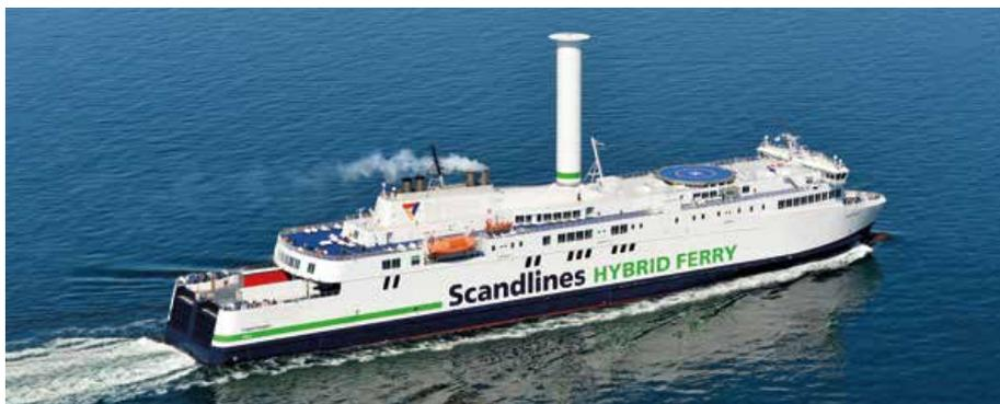
Norsepower Rotor Sails installed on Scandlines' vessel *Copenhagen*
