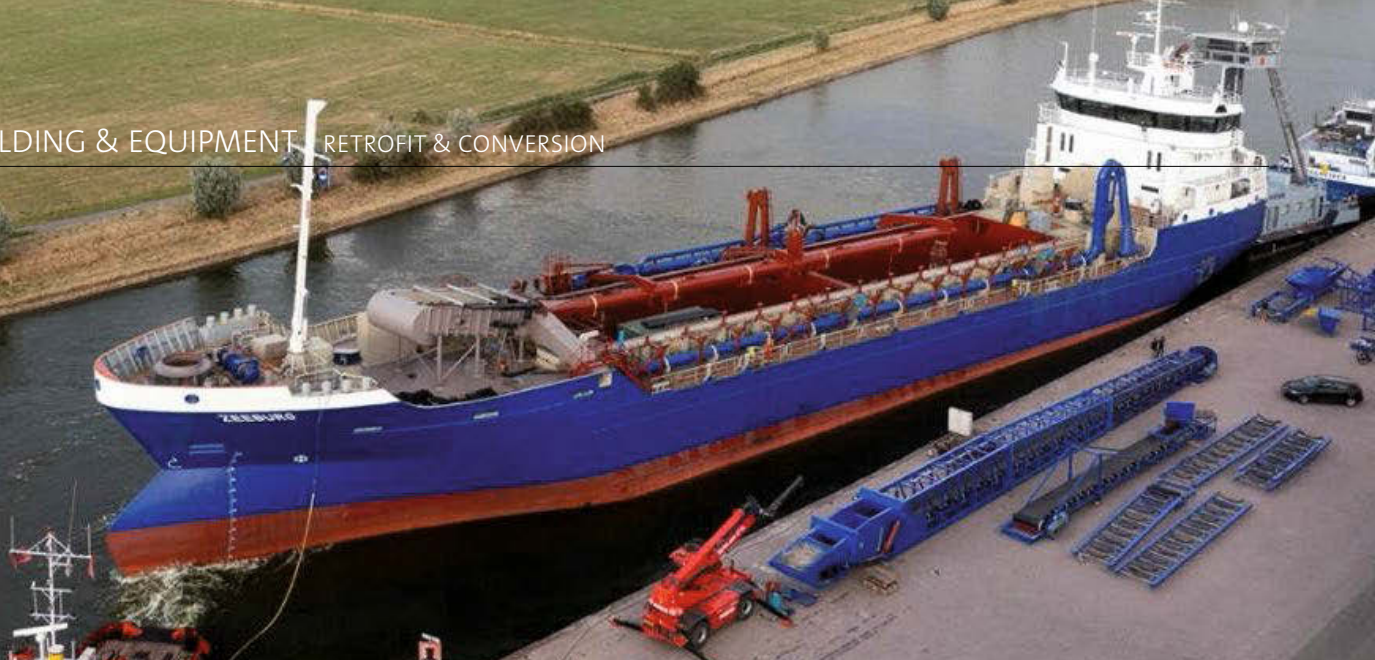
The 90m-long cargo vessel Bente was converted into a TSHD
