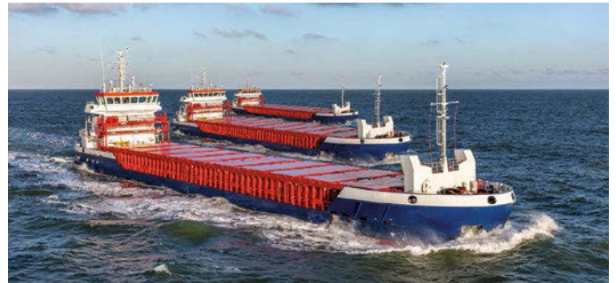
The Combi Freighter (CF) 3850 is a recently redesigned general cargo vessel with a deadweight of 3,850 tonnes Source: Damen
