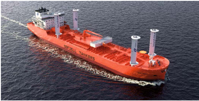
The chemical tanker with bound4blue suction sails Source: Odfjell
