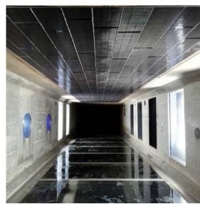
Figure 2: Flat plate setup for friction measurements. Here the surface is covered with AIRCOAT foil.
