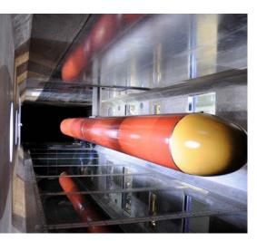
Figure 3: Torpedo-shaped test setup for friction measurements. Picture taken during friction measurements for the AIRCOAT project.
