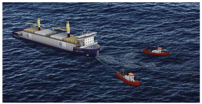
The ship will travel at four knots with the waste plastic collected by two smaller vessels towing a two-mile net that funnels the waste from the surface to a depth of 10m Source: H2-Industries/Technolog
