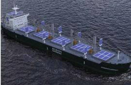
The Aquarius Eco Handymax II bulker design is all electric and is equipped with fuel cells Source: Eco Marine Power
