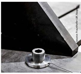
The force-measuring washer based on Delta-C<sup>®</sup> technology from Fraunhofer LBF can be used for monitoring wind turbines
