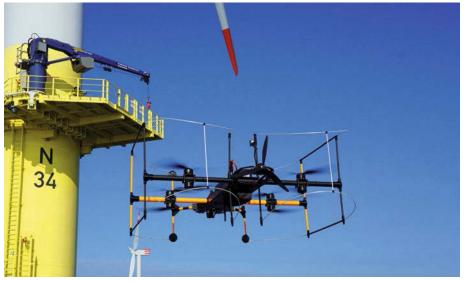
UAS deployment for the inspection of an offshore wind turbine. Supported by the Federal Ministry for Economic Affairs and Climate Action on the basis of a decision by the German Bundestag, Grant: 03EE3057A. Source: Fraunhofer IFAM
