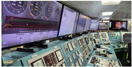
The system is optimised to ensure the best combination for engine RPM and propeller pitch resulting in minimised fuel consumption Source for both images: Qtagg
