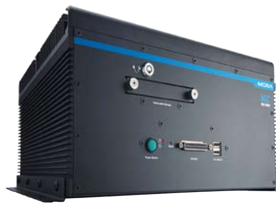
The new x86-based ECDIS computer MC-5157-AC/DC, a high-performance, fanless marine computer. Photo: Moxa Inc
