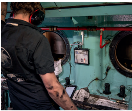
Engine Insights turns onboard cylinder measurement data into clear digital reports on engine condition and wear Photo: Chris-Marine
