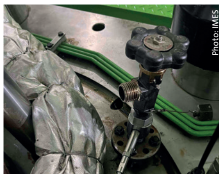
TCS-01CA®-PMI sensor installed on an Everllence ME two-stroke diesel engine
